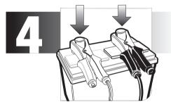
Attach the alligator clamps to the battery. Remember: Red to Positive and Black to Negative. Compressor must be in the off (O) position prior to attaching the battery clamps.
