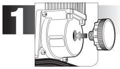
Make sure the intake air filter is installed where the red plug was removed from the intake on the compressor.
