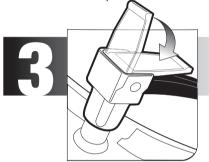
Attach the other end of the 5-in-1 coil hose to the valve stem on your tire.
