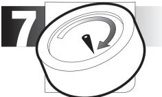
To check tire pressure, manually turn the compressor off. Once the gauge settles, that will be the accurate pressure in the tire.
