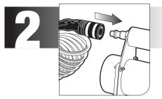
Attach the coil hose to the quick connect coupler on the compressor
